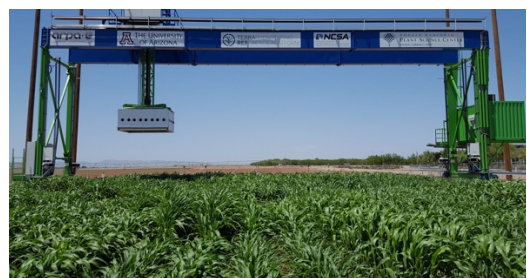
Figure 1: Scanalyzer system (with sensors in white box) operating on 200m steel rails in Maricopa, Arizona.
